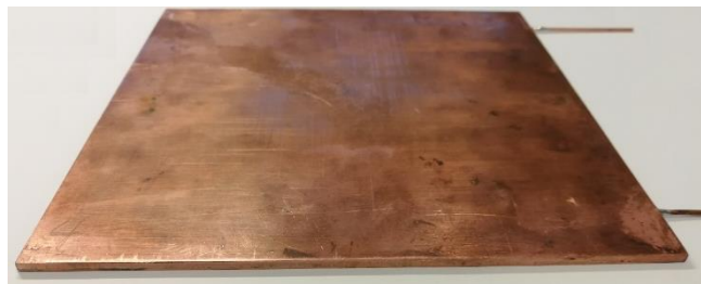
Fig. 4. Vacuum brazed vapour chamber fitted with one feeding line and one line for the pressure transducer.
