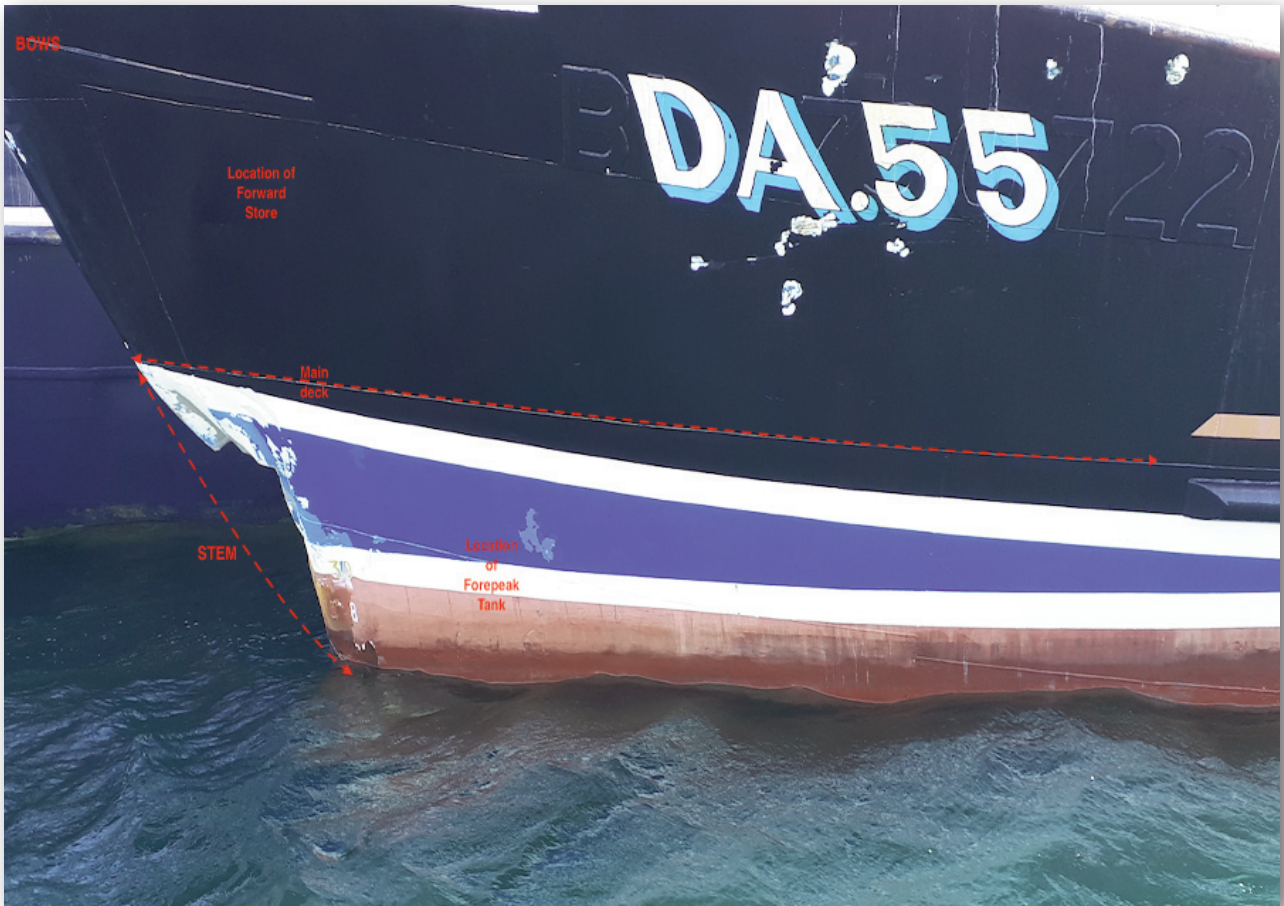
Photograph No.2 - Bow damage above the waterline.
