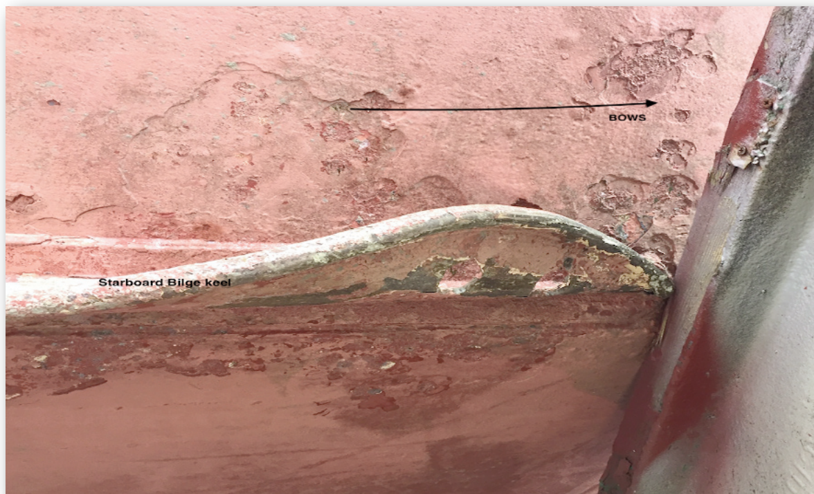
Photograph No.6 - Bilge Keel damage below the waterline.
