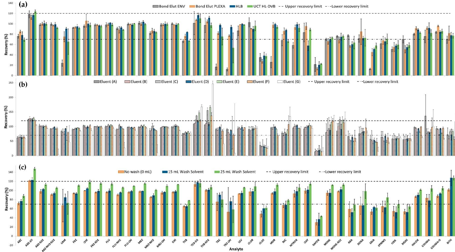
Figure 2-1 Mean recoveries (%) and precision (%RSD, shown by error bars)(n = 3) for assessment of: (a) four different SPE Cartridges (Bond Elut ENV, Bond Elut Plexa, Oasis HLB and UCT HL-DVB) eluted with 50/50 MeOH/MeCN (v/v) (10 mL) (b) seven different eluent compositions: (A) = 50/50 MeOH/MeCN (10 mL), (B) = 50/50 MeOH/MeCN (5 mL) + Acetone (5 mL), (C) = 50/50 MeOH/MeCN (5 mL) + MTBE (5 mL) (D) = 50/50 MeOH/Acetone (10 mL), (E) = 50/50 MeCN/MTBE (10 mL), (F) = 100% Acetone (10 mL) and (G) = 100% MTBE (10 mL) using the HL-DVB cartridge (200 mg, 6 mL) and (c) three different volumes (0, 15 and 25 mL) of water: methanol (90:10, v/v) wash solution using the same HL-DVB cartridge.
