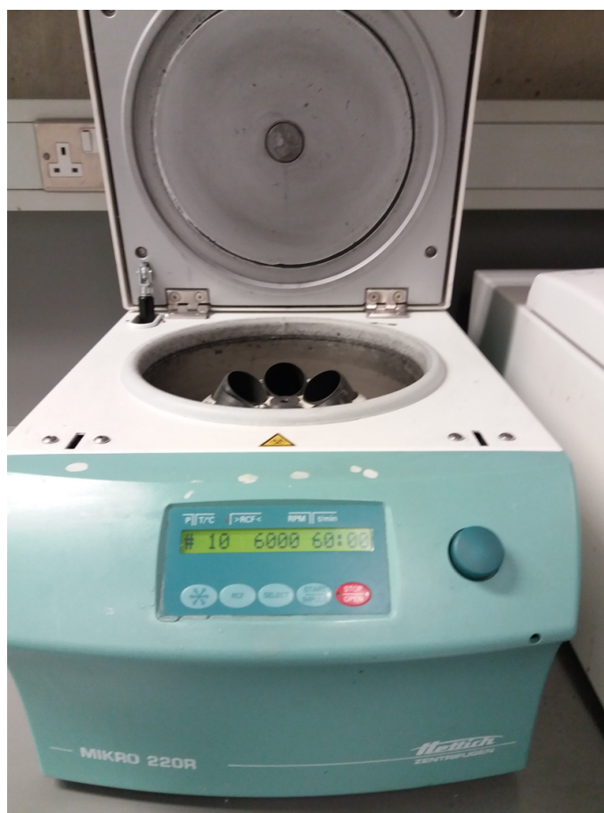
Figure A.1: Hettich Mikro 220R Centrifuge with fixed angle rotor 1016 used for size-selecting LPE samples.
