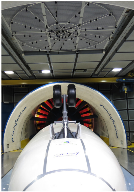
Fig. 3. ALLEGRA NLG model inside the wind tunnel with the top array visible. The view direction is from upstream towards downstream [44].
