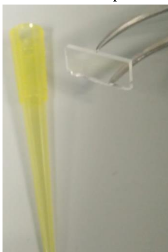
Figure 3.18: LB-Eu-49 monolayer deposited into a 1x2 cm quartz slide.
