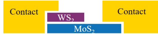
Figure 8.29: Schematic overview of the MoS 2 /WS 2 heterostructure device with asymmetric contacts on the monolayer MoS 2 and heterostack MoS 2 /WS 2
