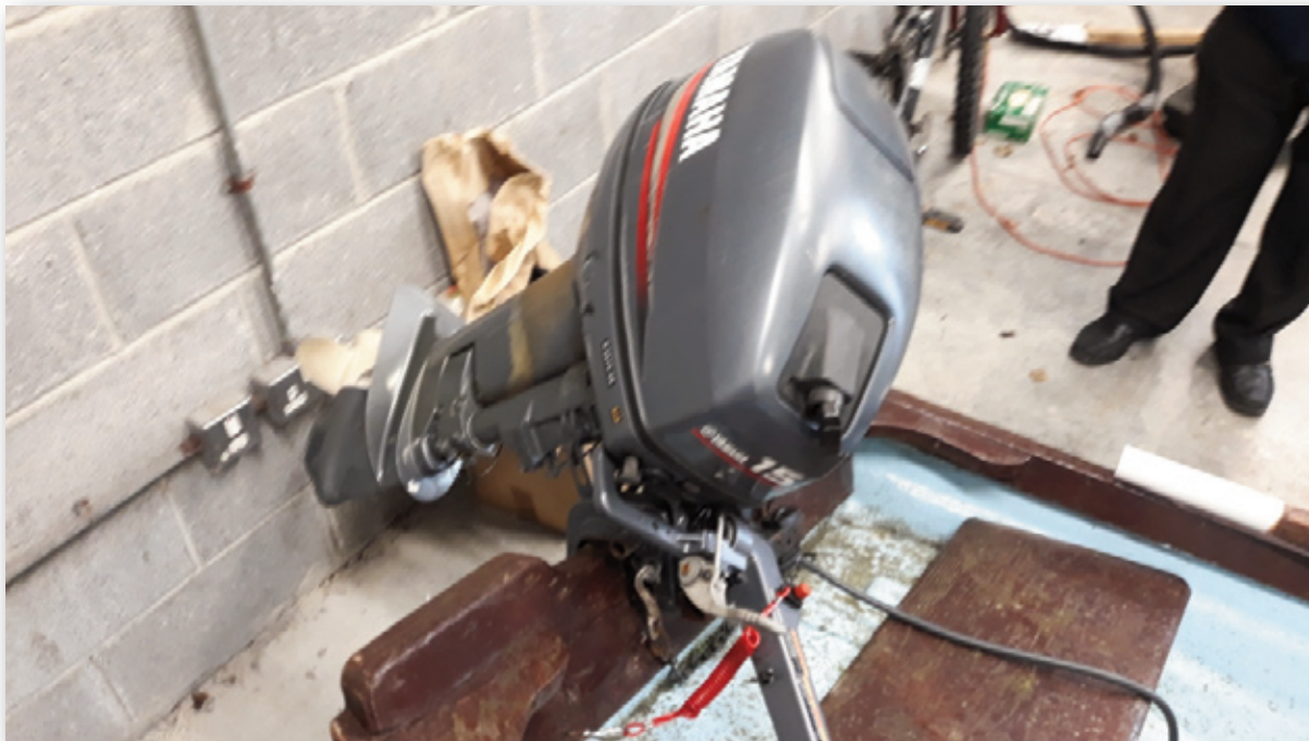
Photograph No.5 - Outboard engine found in gear and kill cord attached to transom.
