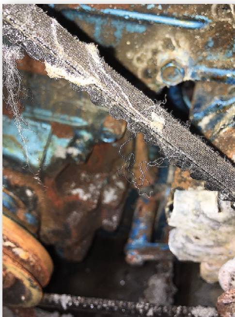
Photograph No.5 - Rust on forward end of starboard engine.
