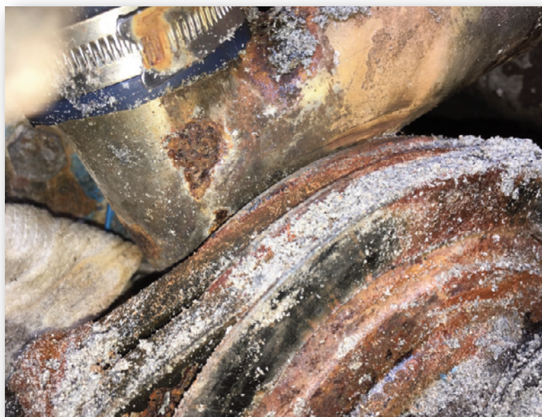
Photograph No.6 - Marks where the water pump drive pulley was in contact with the engine.
