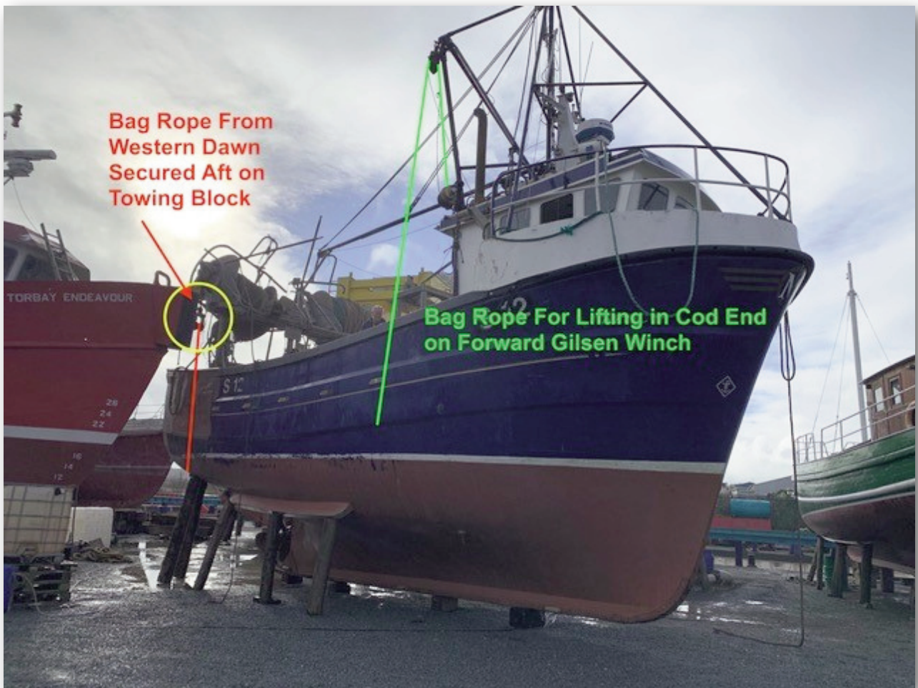
Appendix 7.8 Photograph No. 4 - Hauling Arrangement
