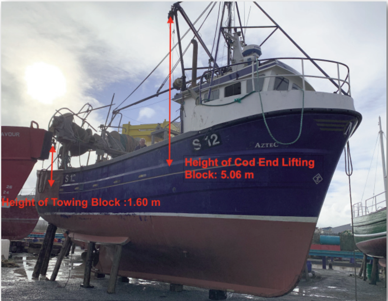
Appendix 7.10 Photograph No. 6 - Lifting Dimensions
