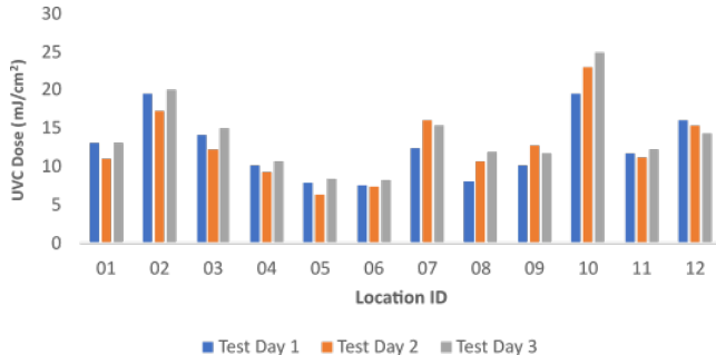
Fig. 5. Graph of the recorded UVC dose at each of the 12 locations over over the course of a UVGI disinfection procedure using the Akara robot.
