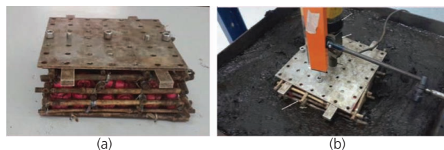
Figure 1. Ultralightweight footing for supporting lightweight structures bearing on peaty ground: (a) model footing comprising of bamboo frame structure incorporating recycled WPB inclusions; (b) vertical load testing of footing in peat bed (taken from Aminu et al. (2022))
