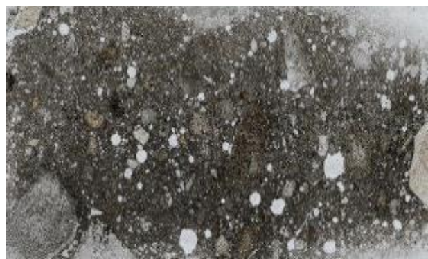
Figure 14. Na 2 SiO 3 + NaOH activated GGBS cured at 60°C shows stronger reaction, a more homogeneous matrix where much of the GGBS has become cement. Scale as in figure 13.
