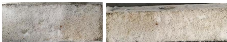
Figure 6 Efflorescence on NaOH activated GGBS after 20 freeze- thaw cycles (left 20°C-cured; right 60°C).
