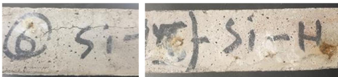
Figure 5 \text{Na}_2\text{SiO}_3 activated GGBS after 25 wet-dry cycles. Left image 20^\circ\text{C} cured, right 60^\circ\text{C} cured showing cracks, delamination and slight efflorescence.
