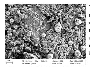
The microstructural (SEM) study of the best performers (Na<sub>2</sub>SiO<sub>3</sub>+NaOH activated, GGBS materials) revealed areas of unreacted GGBS particles bound with scattered silica cements alternating with abundant alumino-silicates. The SEM image (left) shows the isometric and tabular alumino-silicates in the Na<sub>2</sub>SiO<sub>3</sub>+NaOH activated GGBS materials.
