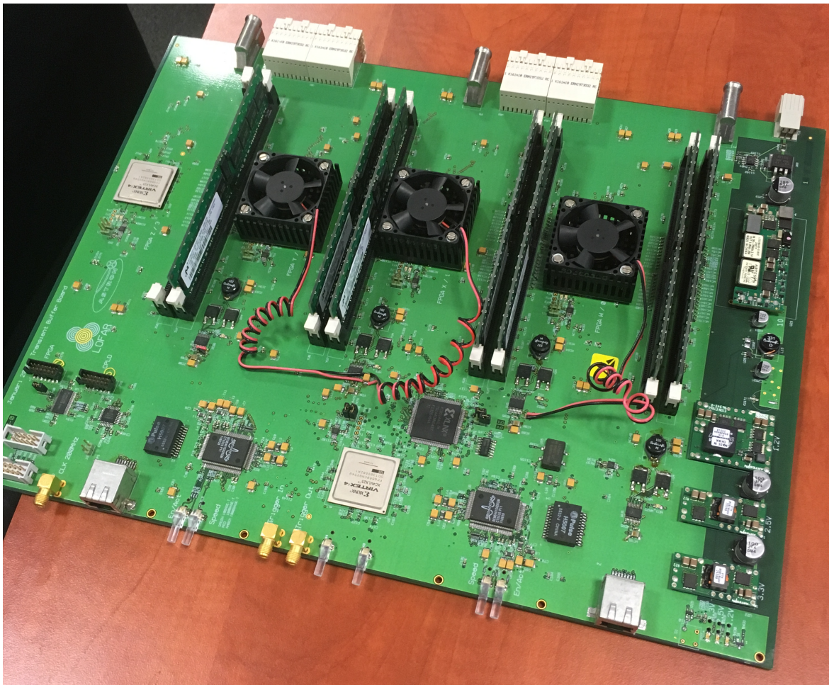
Figure 3.8: A photograph of a Transient Buffer Board taken at the LOFAR data school 2018. This is used to store up to 5 s of raw voltages from LOFAR antennas at 5 ns temporal resolution.
