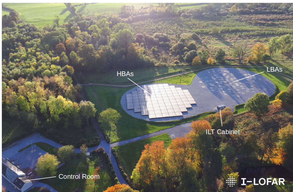
Figure 3.9: Aerial photograph of the Irish Low Frequency Array station IE613 (I-LOFAR) at Birr Castle, County Offaly. Data from the LBAs and HBAs are transferred to the ILT Cabinet (centre right) via coaxial cables where they are amplified, filtered and digitised. In international mode, data are transported to Groningen in the Netherlands at \sim 3.2 Gbps. In local mode, data are processed using REALTA in the I-LOFAR Control Room (bottom left). Image credit: Alison Delaney (Birr Castle).
