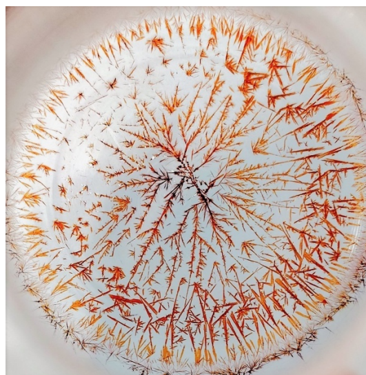
Crystals of photoactive BODIPY dye in pattern spreading as tree branches in a flask
