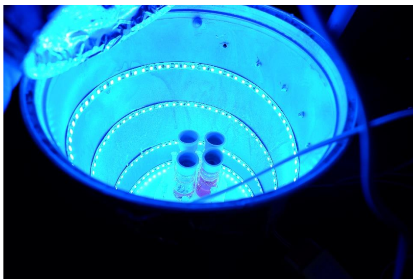
Figure 4.6. The BucketOfBlue ( BoB ) photoreactor.
